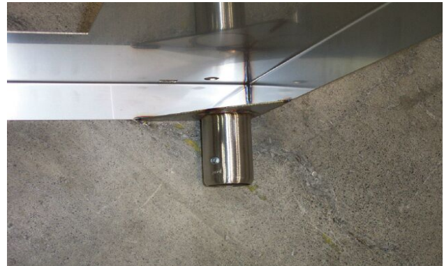
Figure 1—Leg socket showing set screw
