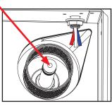
4. Remove sump strainer and pan strainer.
