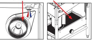
5. Use a hand-scraper to scrape soil and debris into a trash basket.
