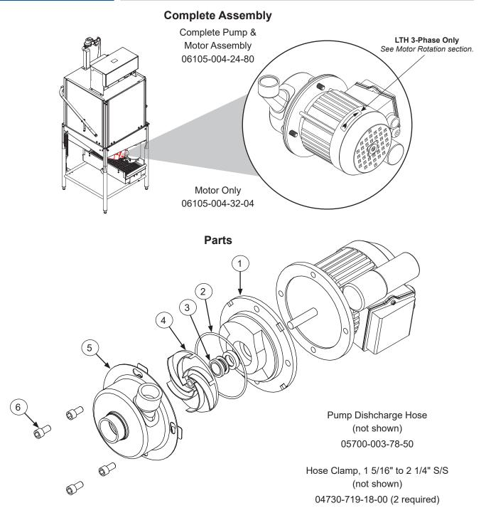
ITEM QTY DESCRIPTION PART NUMBER 1 1 Seal Plate 05700-002-81-87 2 1 Case O-ring 05330-002-81-83 3 Mechanical Seal 1 05330-002-34-22 4 1 Impeller Assembly 05700-002-81-86 5 1 Pump Casing 05700-002-85-01 1 6 Case Capscrew 05305-002-81-88
