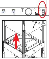
3. Remove drain stopper and allow tub to drain.
