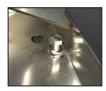
24. Align the edges of the stand with the edges of the dishmachine.
