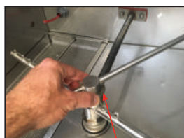
Unscrewing the Wash & Rinse Arms
