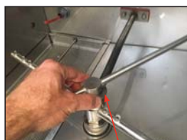
Unscrewing the Wash & Rinse Arms
