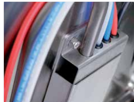
Air gap eliminates possible water leaks
