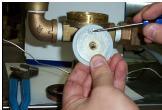
Pointing out the extension hole
