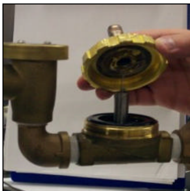
Removing the valve bonnet
