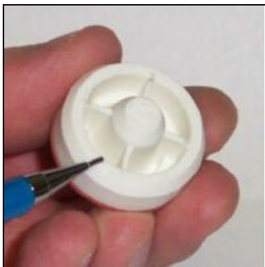
Examining the plunger seating surface
