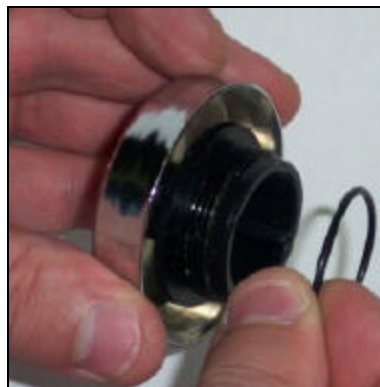
Replacing the O-ring
