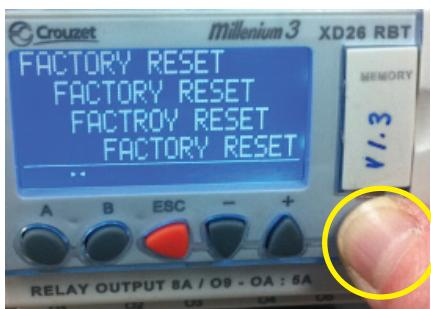
16. Do a quick check: press the "A" key three times and there should be values in the parameters.
