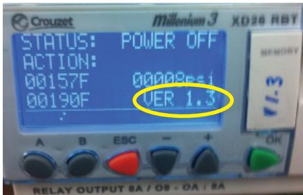
14. Press the "B" key to go to "Reset to Factory" screen.
