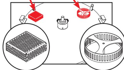
4. Insert middle of bottom wash arm into support bracket.
