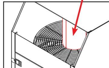
8. Hold paddle switch against wall of machine with one hand.
