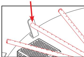
5. Push bottom wash arm onto manifold.
