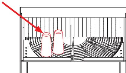
3. When the glasses have completed the cycle, the paddle switch will activate, turning off the water and carousel.
