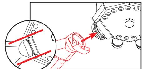
*Align bottom of arm with guide tab on stop cap for easy install.*
