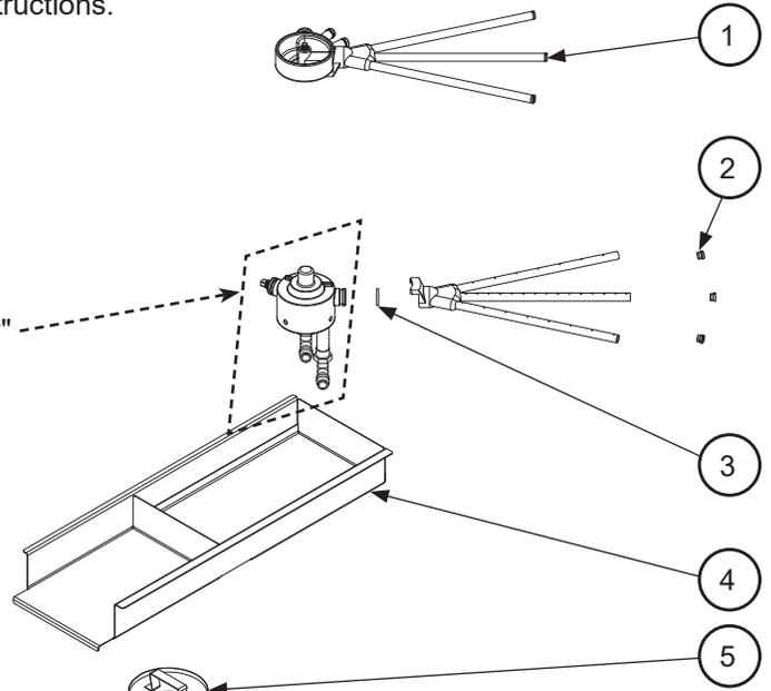
Drain O-ring installs into fitting in bottom of wash tank.
