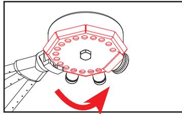
12. Insert middle of top rinse arm into support bracket.
