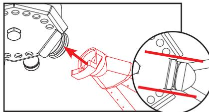
*Align bottom of arm with guide tab on stop cap for easy install.*
