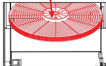
10. Rotate top stop cap counter-clockwise until opening aligns with top rinse arm.
