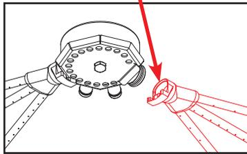
12. Rotate top stop cap counter-clockwise until opening aligns with top wash arm.
