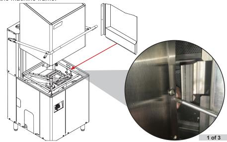
For corners with wall surfaces that are susceptible to water damage, the optional false panel reduces the amount of water hitting the wall whenever the hood is raised.
