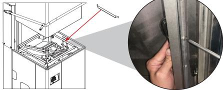
3. If using the false panel, secure the bottom of the panel to the right-side track using hardware from Step 1, and locate the holes at the back of the panel over the studs in the machine frame.
