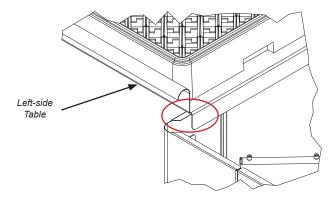
6. Seal each dish table joint with a food-grade sealant to prevent leaks.
