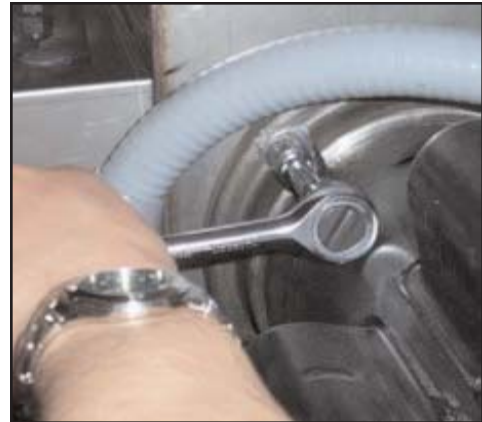
Removing the mounting plate nuts with the 9/16" socket
