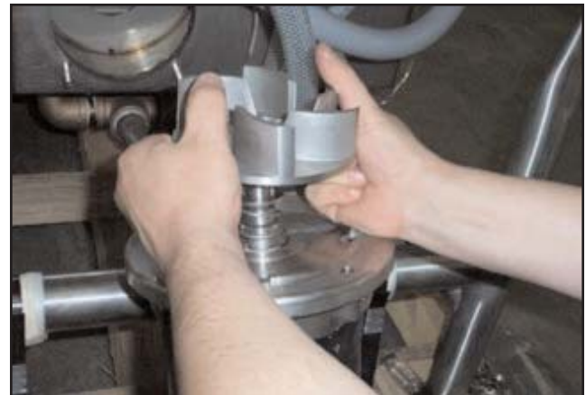
Removing the impeller
