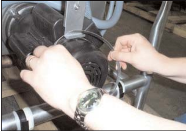
Removing the rear clamp
