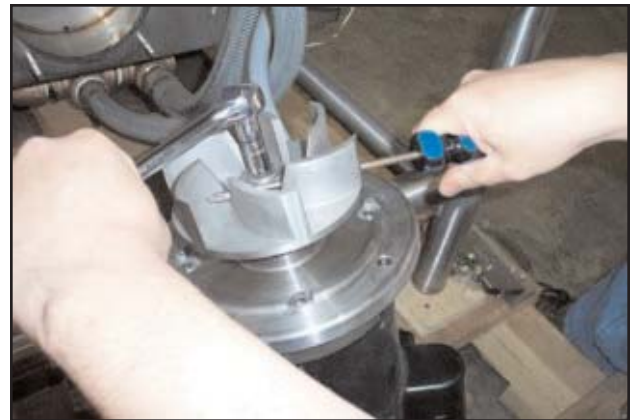
Removing the bolt that holds the impeller to the shaft
