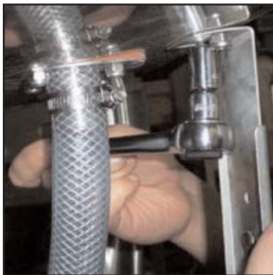
Removing the motor support bracket
