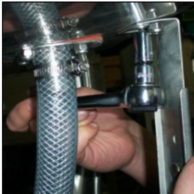
Removing the motor support bracket
