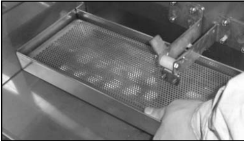
Lifting out the rinse tray assembly
