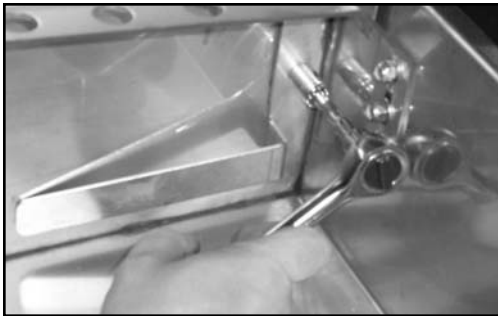
Removing a rinse tray guide bracket
