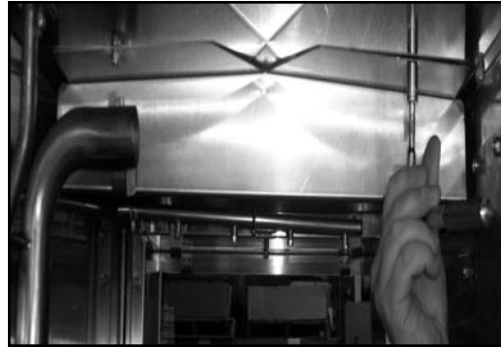
Removing and turning splash shield
