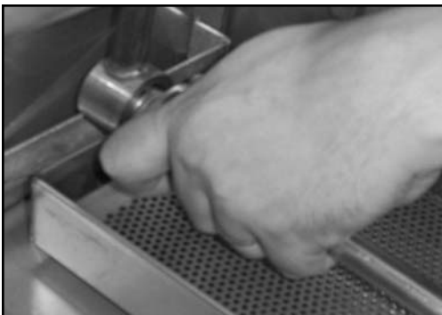
Unscrewing and removing the lower rinse arm
