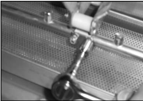
Removing the lower rinse arm support bracket
