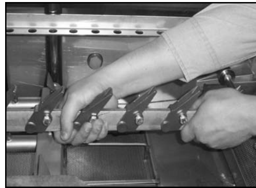
Remove the pawl bar by grasping firmly and lifting up.
