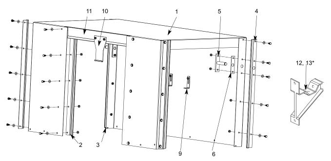
OLD STYLE: If your unit uses items 5 and 6, it is the old style hood weldment. Items 3 thru 6 are used only with the old style Hood Weldment. The hood will have the proper mounting holes in the rear door guides and in the hood itself.
