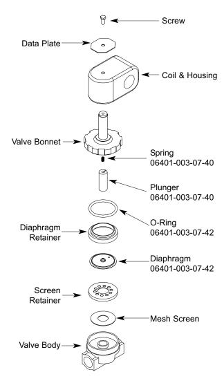
Complete 110 Volt Solenoid Valve Assembly 04810-100-53-00 Coil & Housing only 04810-200-01-18
