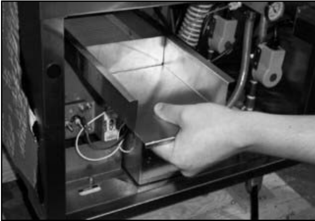
Removing upper (wash) strainer.
