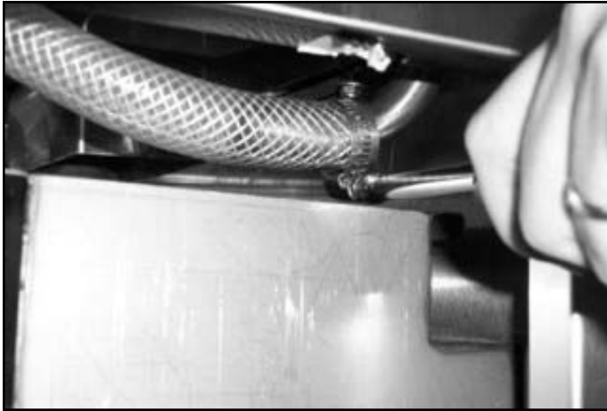
Loosening the discharge hose clamp.
