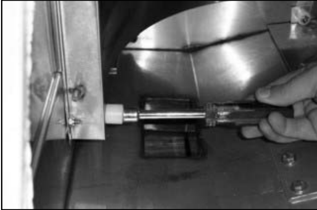
Loosening the roller locknut.
