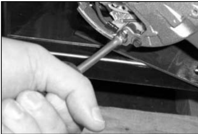
Removing the grounding screw.
