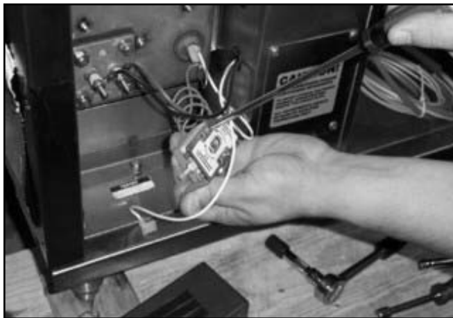
Separating the thermostat from the bracket.
