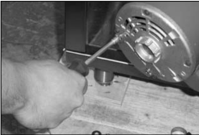
Removing the wiring cover.
