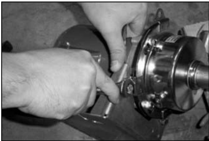
Removing the mounting bracket.
