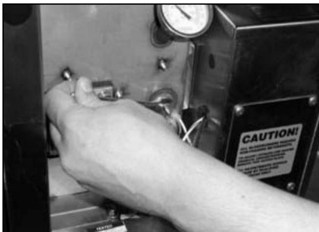
Removing the probe and imperial brass fitting.
