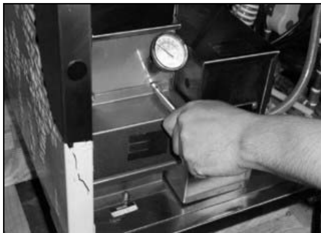
Removing the heater cover.
