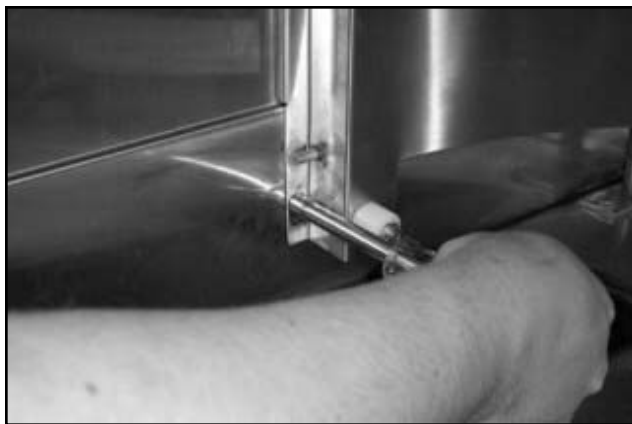
Remvoing the locknuts.
