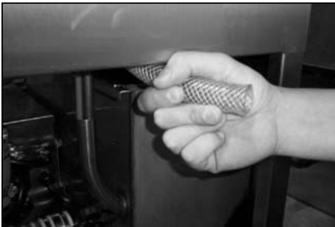
Pulling the discharge hose out.
