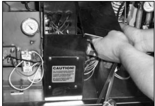
Removing the electrical box cover.
