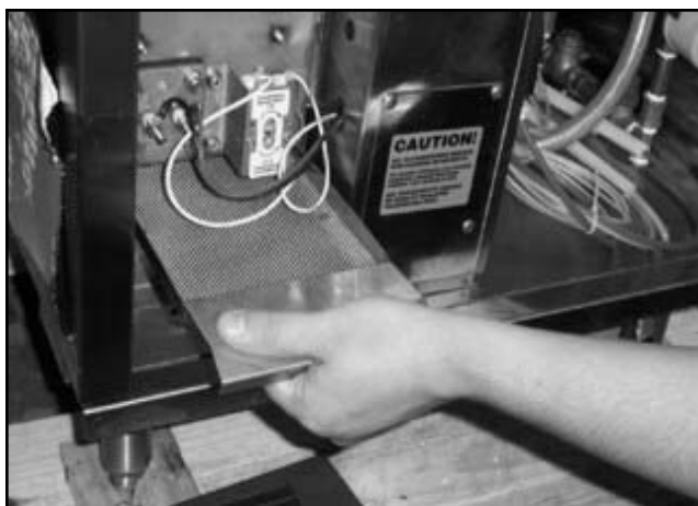
Removing the lower strainer.
