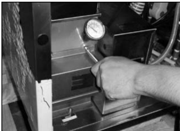
Removing the heater cover.
