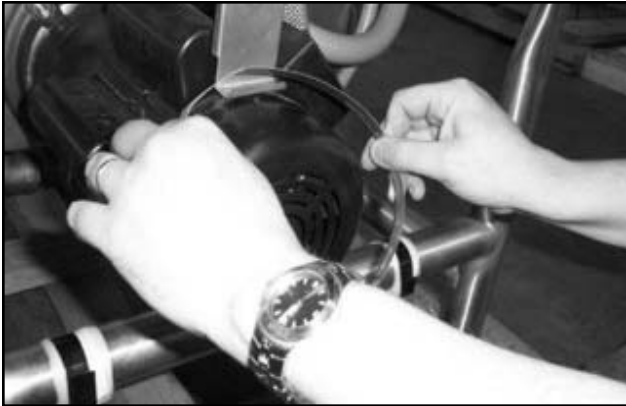
Removing the rear clamp
