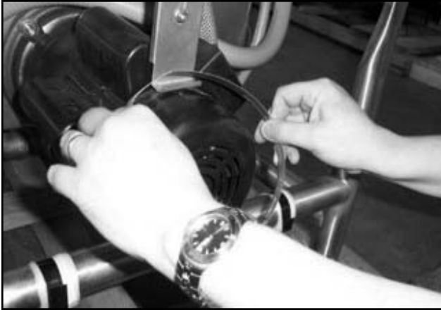
Removing the rear clamp
