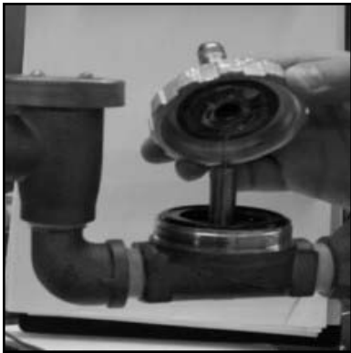
Removing the valve bonnet
