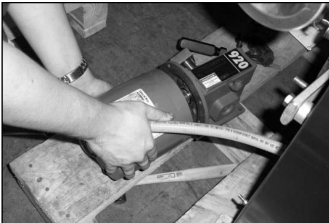
Mounting the motor to the gear reducer.
