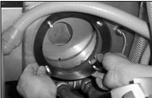
Removing the pump gasket
