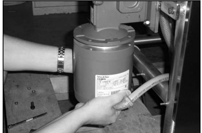
Removing the drive motor.
