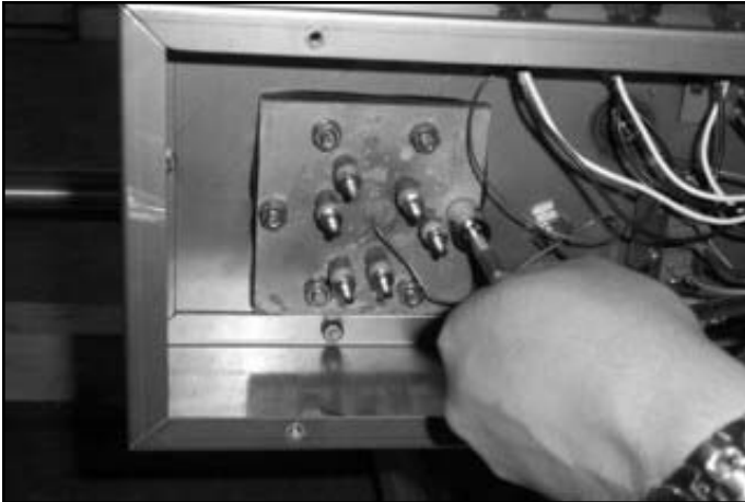
Removing the nuts and lockwashers
