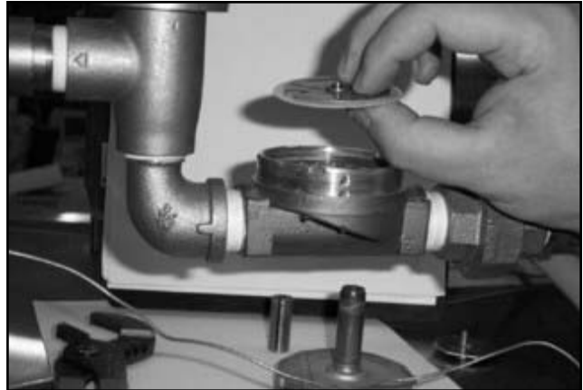
Removing the diaphragm
