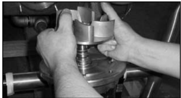
Removing the impeller
