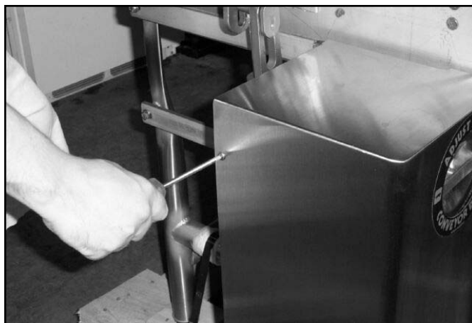
Removing the screws from the top cover.
