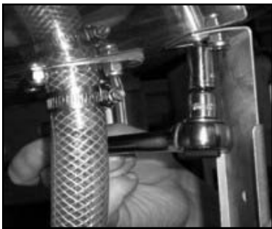
Removing the motor support bracket
