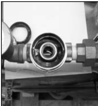
View inside the solenoid valve body
