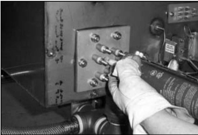
Applying silicone to the heater well
