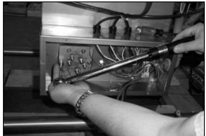
Applying the torque wrench to the nuts
