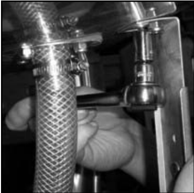
Removing the motor support bracket
