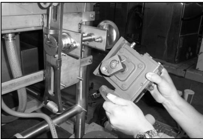
Removing the gear reducer.
