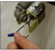
Straightening the wires
