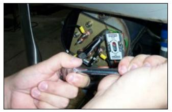
Removing the thermostat bracket/heater nuts.
