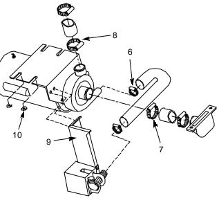
Replacing the Pump Motor
