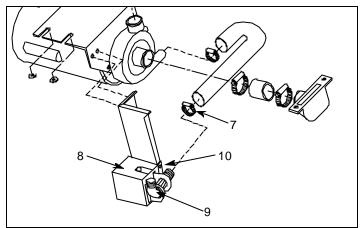
Replacing the Drain Valve
