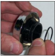
Replacing the O-ring
