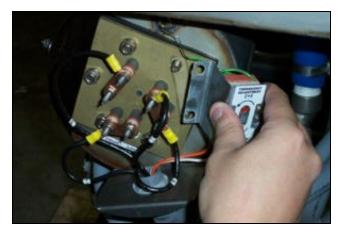
Removing the thermostat bracket.
