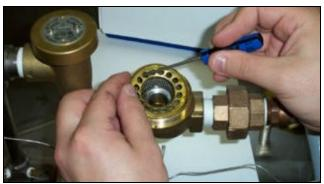
Removing the screen retainer
