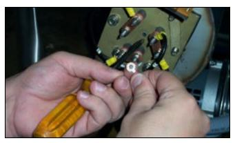
Fitting the jumper into the mounting cup.
