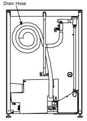
Back of Machine Showing Drain Hose
