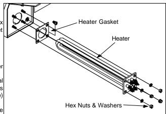
Replacing the Heater
