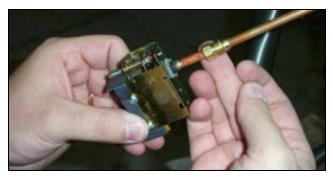
Sliding imperial fitting onto new thermostat.
