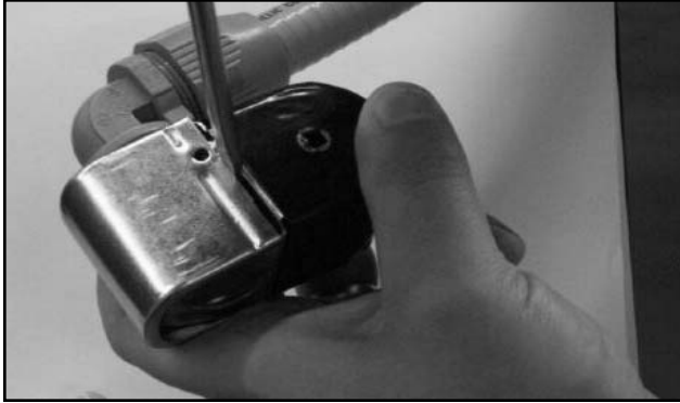
Prying open the coil wire cover
