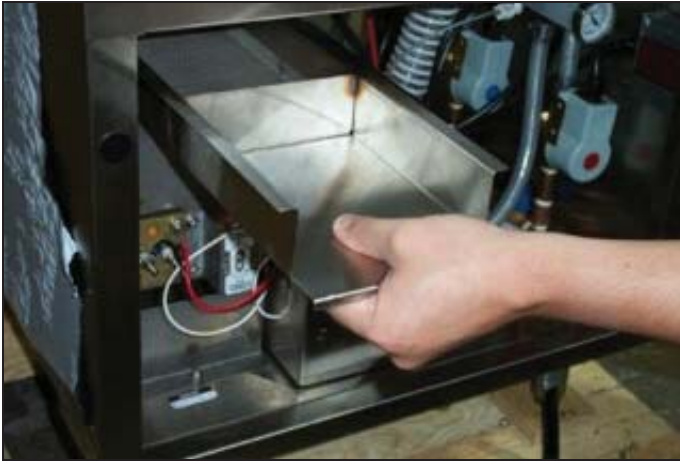
Removing upper (wash) strainer.
