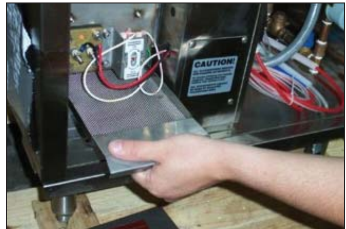
Removing the lower strainer.
