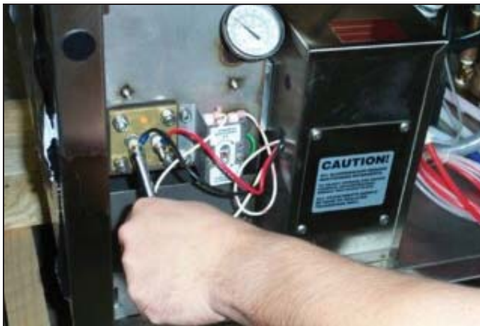
Removing the heater nuts.
