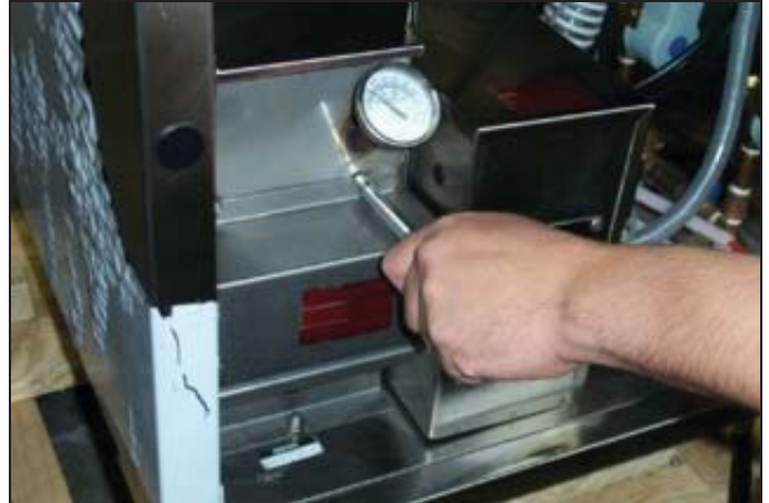
Removing the heater cover.
