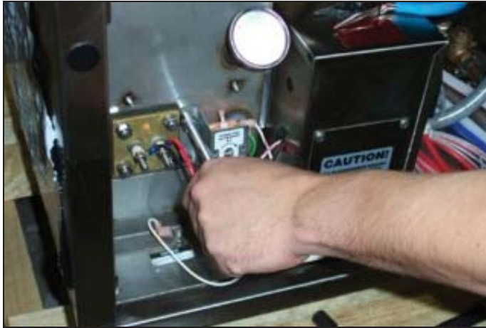
Removing the thermostat bracket mounting nuts.
