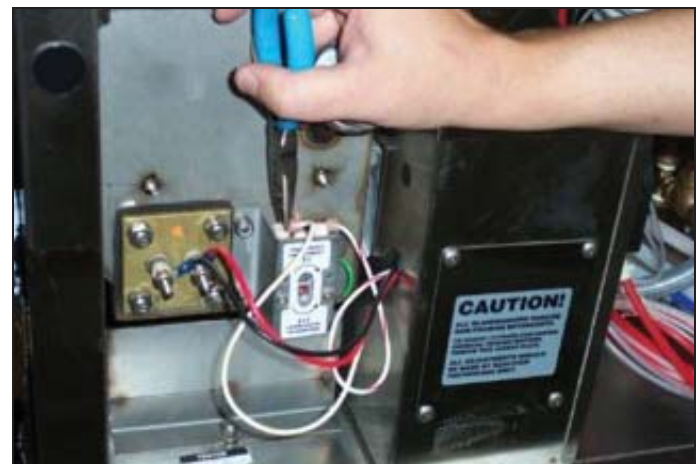
Removing the terminals.
