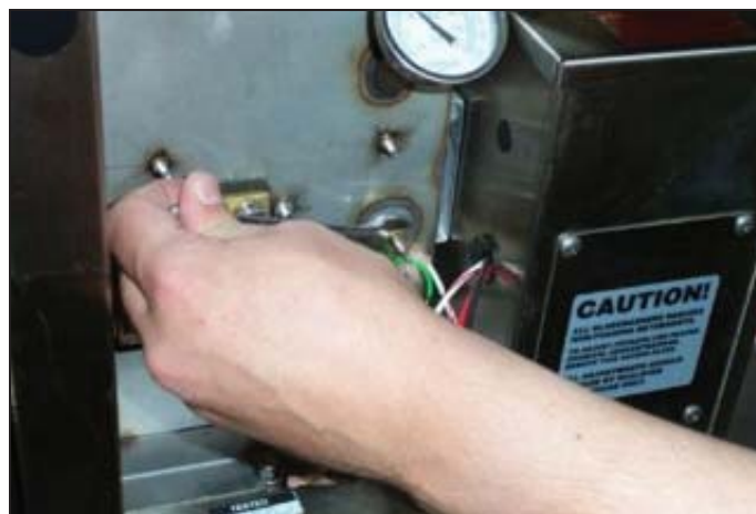
Removing the probe and imperial brass fitting.
