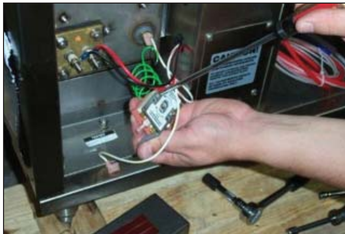
Separating the thermostat from the bracket.
