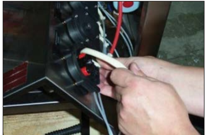
Pulling the rubber tube out of the pump.
