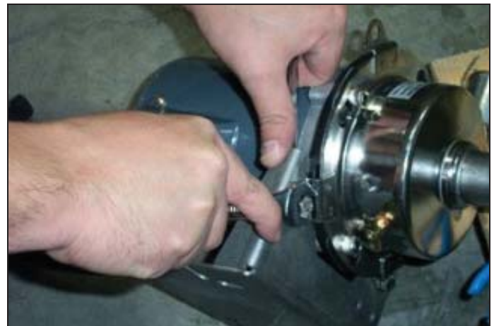
Removing the mounting bracket.
