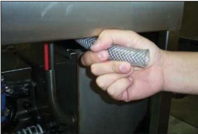
Pulling the discharge hose out.
