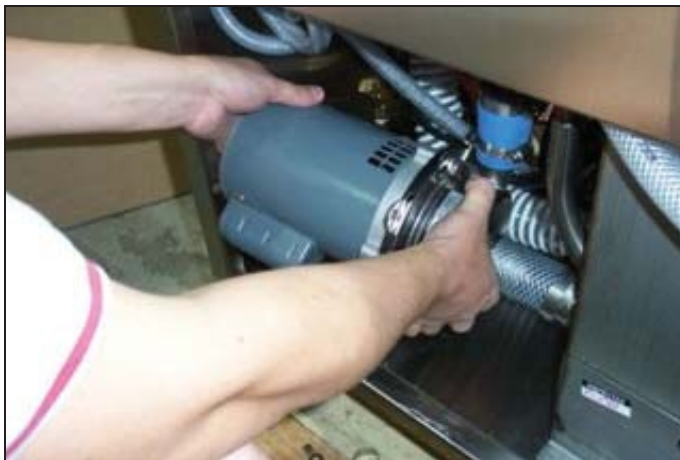
Lifting up on the motor.
