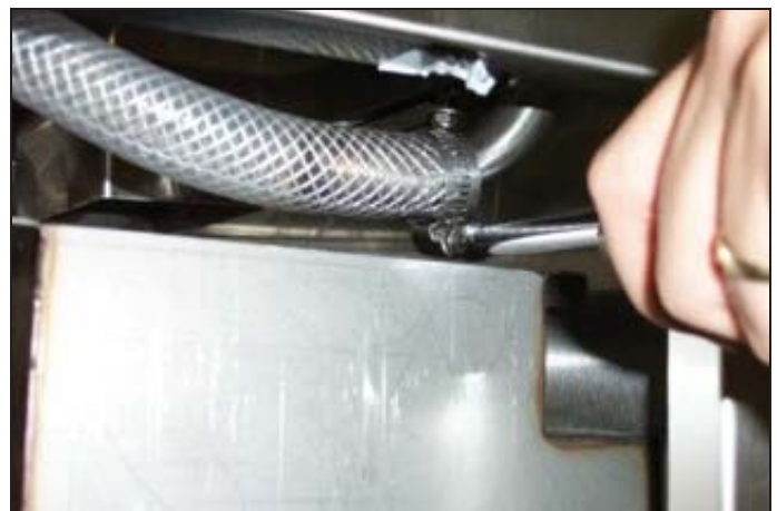
Loosening the discharge hose clamp.
