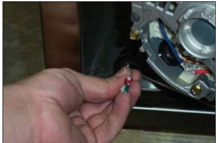
Removing the power wires.
