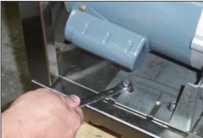
Removing the assembly mounting nuts.
