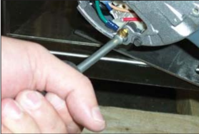
Removing the grounding screw.
