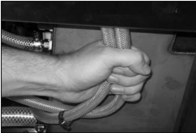
Pulling the discharge hose out.
