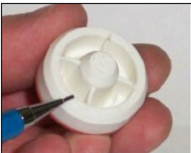
Examining the plunger seating surface
