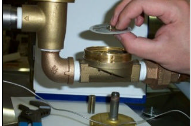
Removing the diaphragm
