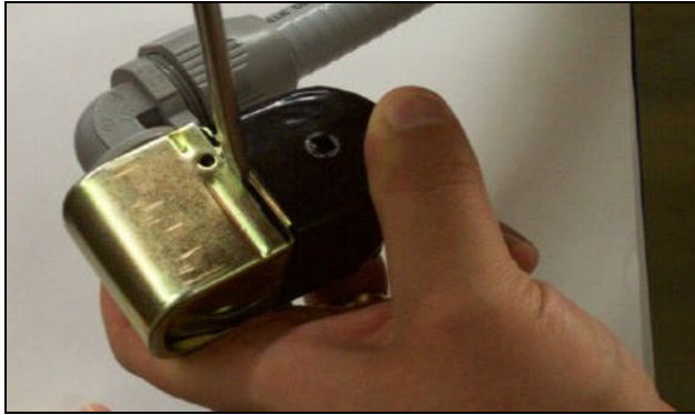
Prying open the coil wire cover
