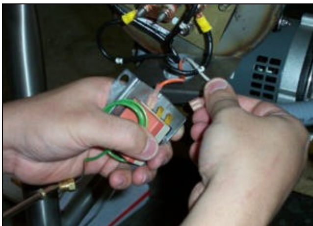
Removing the wires from the thermostat.
