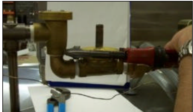
Loosening the valve bonnet
