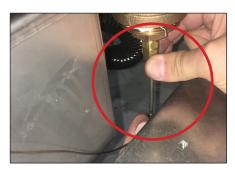
21. Take the conduit and wires coming from the solenoid coil and run the wires through the fitting (05975-011-45-14) on the bracket and connect the conduit to the back of the fitting.
