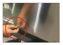
Take the Wash Tank Heater Cover off. Discard the cover and keep the hardware.
