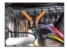
16. Run the other end of the SJ cord under the wash tank and through the hole in the back of the bracket (05700-004-39-53).
