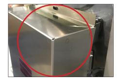
4. Remove the four bolts holding the control box to the frame (right side shown) and keep the bolts.
