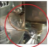
19. Loosen nut and ferrule on assembly 05700-004-14-96 and insert the thermostat probe into the compression fitting. Insert the length of probe shown below.
