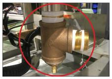
7. Install Tee (04730-011-69-93) and Elbow (04730-206-32-00) onto the assembly installed in the last step. Make sure middle opening on the tee is parallel with bottom of wash tank. Turn the assembly so it is inside the machine.
