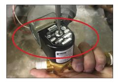
9. Install assembly 05700-004-14-95 to the middle opening on the tee installed in Step 7.
