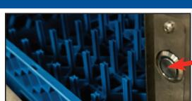
4. Open door and add amount of deliming solution recommended by chemical supplier.
