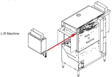
3. Install the drip tray underneath the top coil support and secure it and the Energy Recovery System to the top coil support using the washers and nuts provided.
