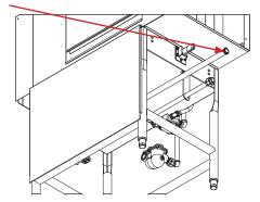
4. If a steam blower dryer, connect the plumbing to the dishmachine and put the solenoid valve top on.
