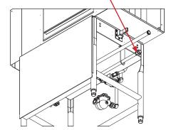
5. Connect wiring to the back of the control box on the dishmachine by joining like colors.
