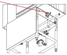
3. Connect the drain line to the dishmachine.
