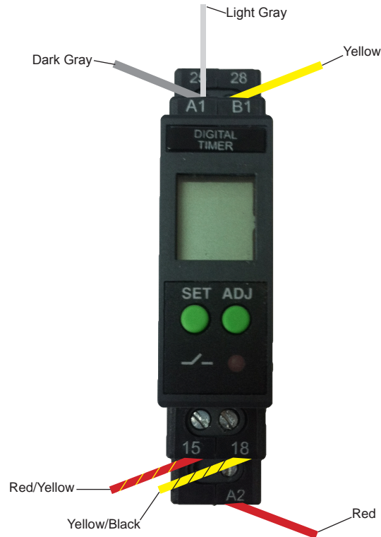
Timer Wiring with Correct Wire Colors
