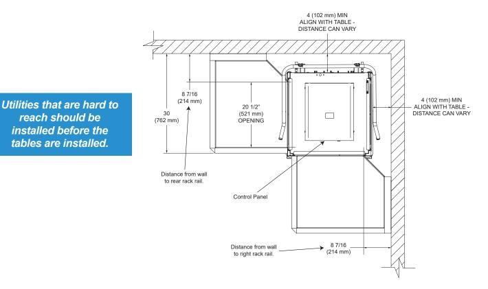
2. The dishmachine must be located so the dish tables and the rack rails in the dishmachine align for proper loading and unloading of dish racks.
