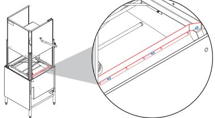
3. If using the false panel, secure top of the panel to the right-side of machine hood using the two slots on the panel, then secure bottom to the track assembly.
