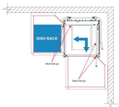
The dish tables are stationary, so the dishmachine must be moved until the rack rails line-up with the proper locations on the dish tables. As a result, distances from the wall might vary.
