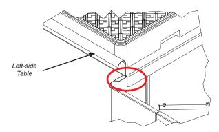
4. Seal each dish table joint with a food-grade sealant to prevent leaks.
