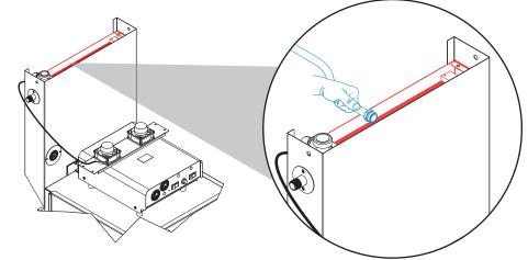
4. If there is scale build-up on the coils, a coil cleaner approved for use in food-process applications must be used. Spray the coil cleaner on the coils until they are saturated.
