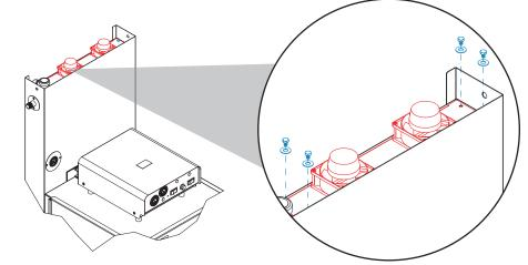
2. Lift the fan mounting plate off of the VER system and set it on the control box, being careful to allow enough slack in the fan wiring.
