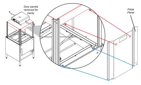
4. Remove and discard the front dress panel to allow access for service (very difficult to remove after tables are installed). Slide up and lift up and out.
