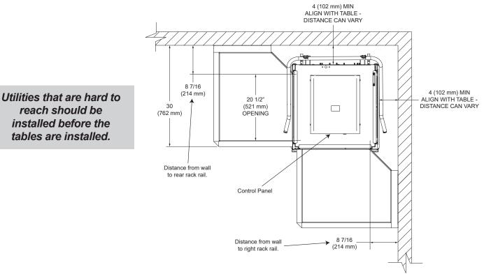
2. The dishmachine must be located so the dish tables and the rack rails in the dishmachine align for proper loading and unloading of dish racks.
