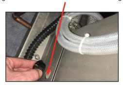
8. Push loose end of the hose through the bushing and push until there is no slack left in the hose (hose can be trimmed, if necessary).
