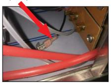
27. Connect black wire to an empty post on top terminal board. If no open post, remove one black wire from terminal board and connect to black wire on Item #3 from kit, using piggyback terminal on wire. Connect to post where black wire earlier in the step was originally connected.
