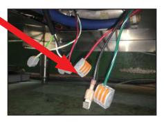
23. Disconnect green/white and black wires from machine 2-way gray/orange splicing connector and connect them to the 3-way gray/orange splicing connector at the end of green/white wire on Item #3 from kit.
