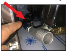
16. Attach drain hose removed in Step 3 to front of stainless steel elbow. Use 5/16 nutdriver/socket or flathead screwdriver to tighten clamp.
