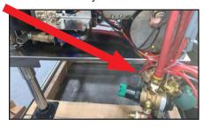
10. Route end of blue hose on Item #1 through hole in machine stand and under wash motor.
