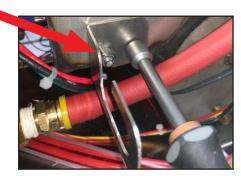
18. Using adjustable wrench, re-install solenoid valve assembly.
