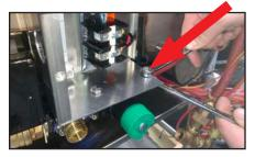
9. Push wires and tubes out of the way.
