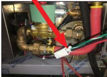
22. Route wires under machine and through hole in machine stand.
