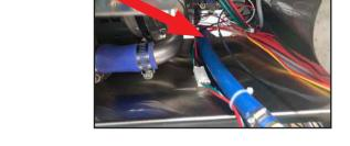
11. Orient 05700-004-60-53, drain water tempering assembly (Item #1 from kit), as shown below. Rotate assembly down and to left and push under terminal box and edge of rinse tank. Then place holes in assembly bracket over studs freed in Step 7.
