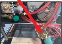
7. Using 7/16 nutdriver/socket, remove plumbing support bracket.
