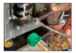
20. On machine, locate 2-way gray/orange splicing connector with a green/white wire and black wire (trace thick black wire from drain valve, will come out of that). Pull wires down through hole in machine stand.
