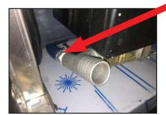
15. Using 1/4" nutdriver/socket or flathead screwdriver, tighten mini-clamp.
