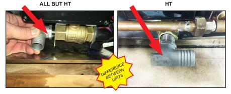
7. Orient drain water tempering assembly from kit as shown below. Push box of assembly under terminal block box (if HT, from side of machine) and push end of red hose under wash motor and out near the drain valve assembly.
