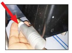
9. Put mini-clamp from kit on end of red hose and orient clamp so it can be tightened later. Install hose onto barbed end of fitting installed in Step 8.
