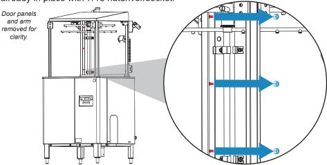
4. Orient false panel as shown below and secure to inside of left hood support using slot on side of panel.
