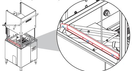
3. If using false panel, locate three studs at back-left of machine and remove nuts already in place with 7/16 nutdriver/socket.
