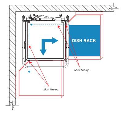
The dish tables are stationary, so the machine must be moved until the rack rails line-up with the proper locations on the dish tables. As a result, distances from the wall might vary.
