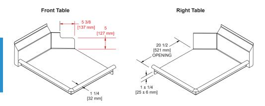
3. For proper loading and unloading of dish racks, locate the machine so dish tables and machine rack rails align.
