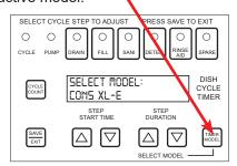
2. Select correct model using ARROW buttons under STEP DURATION.
