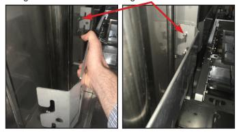
3. The RackStar 44 has one long ware guide and the RackStar 66 has one long and one short. Both ware guides install the same way.
