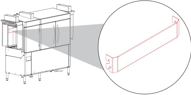
2. Slide the open slots on the ware guide down onto the ware guide studs.
