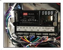
4. Remove old I/O module using phillips screwdriver.
