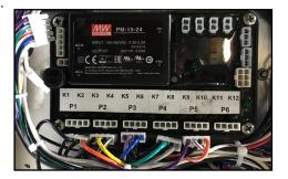
6. Remove old I/O module using phillips screwdriver.
