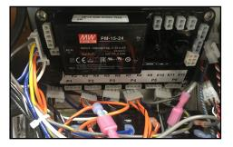
5. Remove old I/O module using phillips screwdriver.
