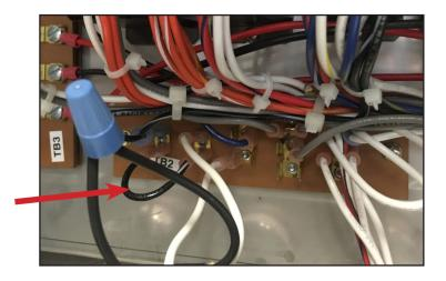
The switch is wired common and normally-open because of the hinge design. By interrupting the line in series with the door switch(es), the dishmachine ceases to operate. Refer to the schematic for details.
