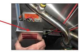
14. Crimp terminals from the kit on the black and white wires from the drain water tempering box.
