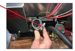
8. Place the bottom of the drain water tempering tube into the top of the 12" hose from the kit.
