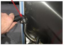
11. Tighten the clamp, ensuring the drain hose is oriented as shown.
