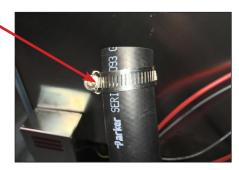
5. Place the 12" hose from the kit where the drain hose was located.
