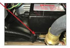
3. Remove the drain hose, keeping the clamp on it.
