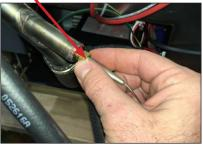
20. Tighten the thermostat fitting with a 7/16" wrench.
