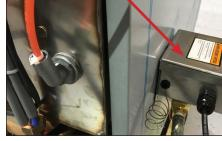
NOTICE 1/4" holes can be drilled in machine panels to mount the drain water tempering box.
