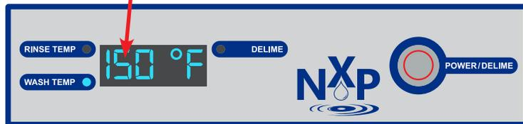
2. Once button is released, each press and release of button fewer than three seconds will advance wash temperature one degree at a time to a maximum of 170 °F, and will then roll over to 150 °F and advance up again.
