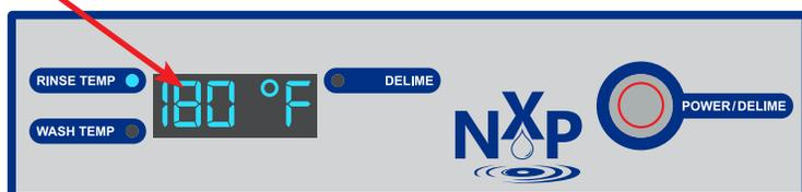
2. Each press and release of button fewer than three seconds will advance wash temperature one degree at a time to a maximum of 192 °F, and will then roll over to 180 °F and advance up again.
