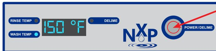
4. To exit setpoints at any time, hold button for a minimum of six seconds. Display wash temperature will stop flashing. The machine is ready to operate.
