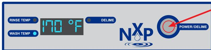
3. Once desired temperature is selected, press and hold button for a minimum of three seconds and no more than six seconds (after three seconds wash temperature will stop flashing). Release button to accept and move to next setting (rinse temperature).
