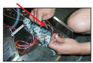
6. Turn the cover over and using the phillips screwdriver, remove the cover to the pump requiring a motor change.
