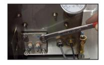
1. Place the heater wires on the heater and tighten the nuts down using the 3/8" nutdriver (Step 7 in reverse).
