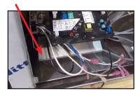
2. Remove the ELAN thermostat using a phillips screwdriver. Either unplug the wires or cut the wire-tie and let the thermostat hang down out of the way.
