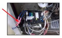
4. Unplug all of the terminals/wires connected to the ELAN thermostat.
