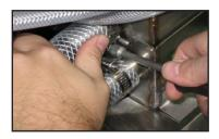
3. Using the same nutdriver, loosen the disharge hose where it connects to the tub weldement.
