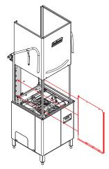
6. Install front rack rail removed in Step 1 on left side of machine, ensuring studs on rack rail go through holes in bottom of false panel.
