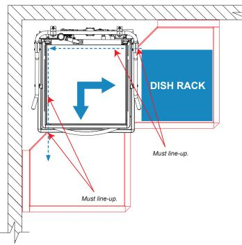
3. Install dish tables so edge of each table fits over inner wall of machine tank.
