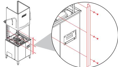
4. Use 7/16 nutdriver/socket to remove two nuts placed for false panel option.
