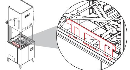
3. If installing false panel, use 7/16 nutdriver/socket to remove three nuts securing rear door track cover at back-left of machine. Discard rear door track cover.
