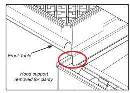
4. Seal each dish table joint with food-grade sealant to prevent leaks.
