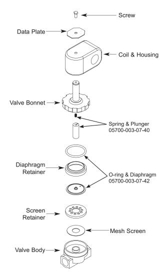
Complete 115 Volt Solenoid Valve Assembly 04810-100-53-00
