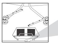
3. Verify the drain stopper is preventing the wash tub water from pouring out excessively. There might be some slight leakage from the drain hole. Verify that there are no other leaks on the machine before proceeding any further.
