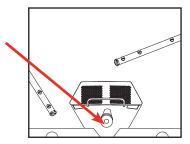
4. Wash tub must be completely filled before operating the wash pump to prevent damage to components. Once wash tub is filled, the machine is ready for operation.
