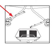
**POWER UP** To place the machine in standby, flip the "OFF/ON/FILL" switch to the ON position.
