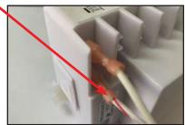
11. Connect other end of white/red harness with piggyback terminal to bottom terminal post on sanitizer prime switch.
